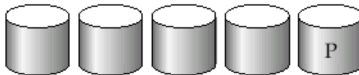
(e) RAID 4: block-interleaved parity
