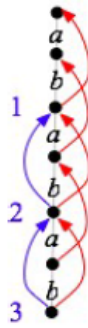
Figure 6: Output links (blue) and failure links (red) for patterns ab , abab , ababab .
